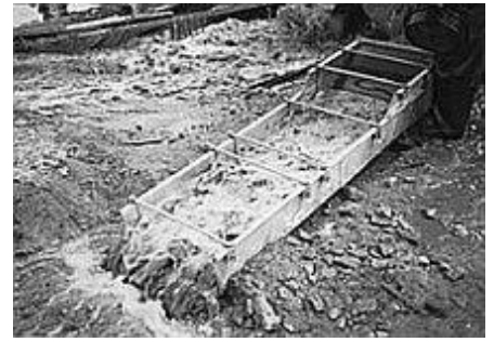
A sluice box used in placer mining
